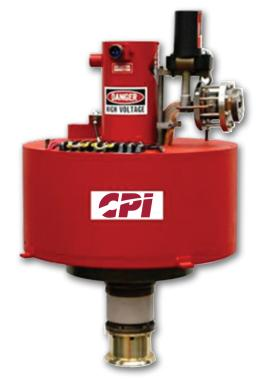
The VKX-8253A is an electromagnet focused, 9.3 GHz klystron which has demonstrated peak power of 5.5 MW with 18 kW average, at an RF pulse width of 2.5  $\mu$ s. The klystron achieved power of 6 MW peak at 6 kW average. The unit was designed to achieve 20 kW average power at 5 MW peak.
